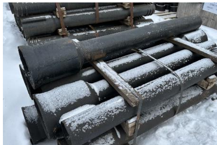
A Valve Box Bottom Section (Cast Iron)
