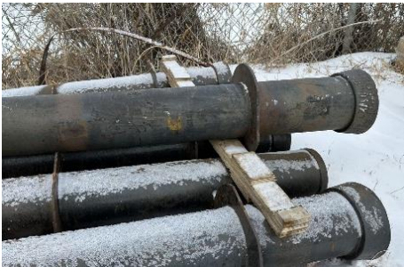
A Valve Box Top Section (no threads, sliding type)
