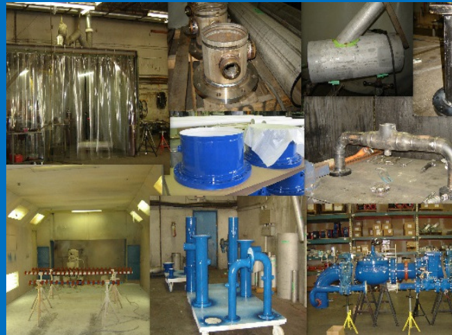
L-R: Stainless Steel Isolation Booth, Pipe Spools in Various Stages of Fabrication, Couplings in Our Paint Booth Waiting to be Coated, Pipe Spools in Our Drying Area, PRV Station in Assembly
